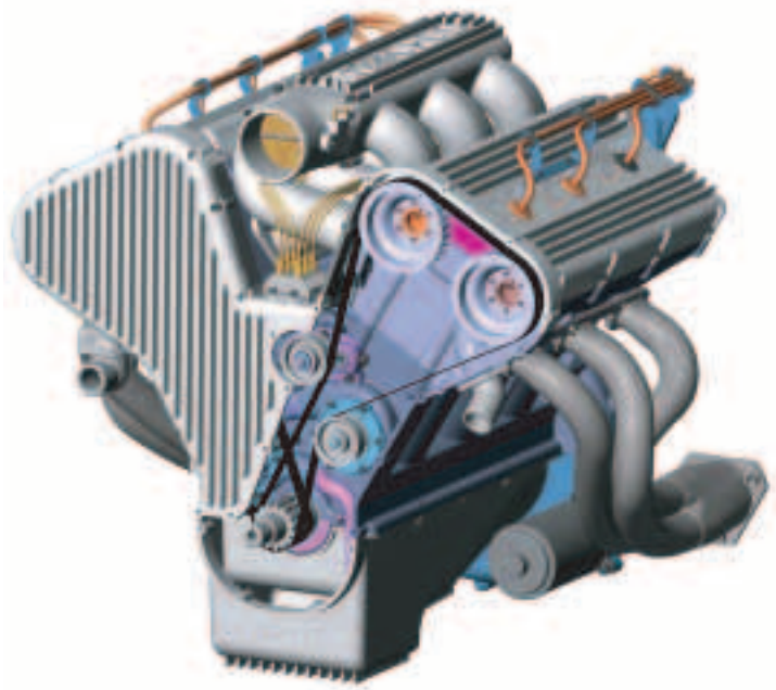
FIGURE 1.28. An assembly model of an Omnica 3.2-liter V-6 engine made from a collection of solid model parts.
