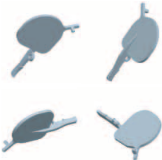
FIGURE 1.27. Solid modeling allows a proposed part to be easily visualized in a variety of orientations.
